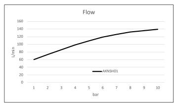
Water consumption at fully opened nozzle, depending on pressure
